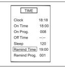
3. Press the CH+/- buttons to move the indicator to "Remind Prog. ", then press the VOL-/+ buttons to adjust (For example, 18).
